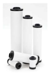
We use high efficiency borosilicate glass microfibre media to remove all dirt particles. All elements include stainless steel metalwork and are fitted with an external pre filter layer of 80 p.p.i., open cell reticulated polyester foam. These filters are a proven success and now include such features as differential pressure indicators which are a specific requirement of the HTM02-01 medical gas pipeline specification.
